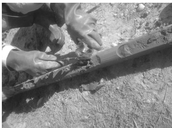
Fig.4 Prelevare probe sapa tip side window
